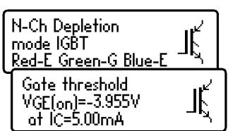
The **DCA Pro** can drive the gate from 0V to -5V for depletion mode IGBTs.
