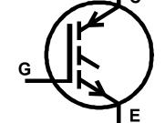
It combines the input characteristics of a MOSFET with the output characteristics of a Bipolar Junction Transistor.
