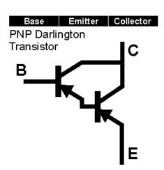
Note that the component schematic is displayed in colour to illustrate which colour test lead is connected to each component lead.
