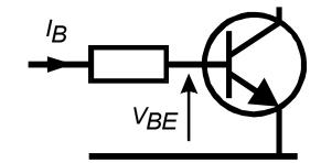
VBE=0.703V at IB=5.00mA This example shows an NPN base-emitter voltage ( $V_{BE}$ ) of 0.703V for a base test current ( $I_B$ ) of 5mA.
