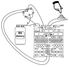
USE A SLIDE SWITCH (ON OFF ON)
