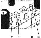
Make sure to put a 1A T (slow-blow) fuse in series with the primary winding
