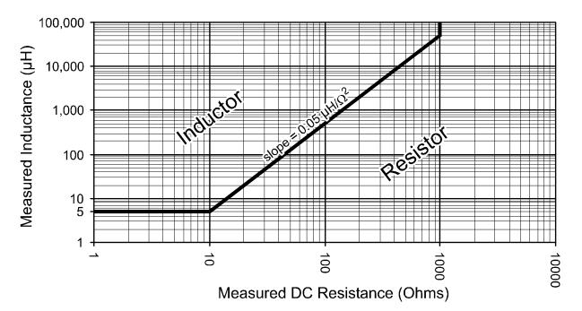
For example, if the inductance of your component is measured at  $100\mu$ H and it has a DC resistance of  $100\Omega$ , then the Atlas LCR will tell you that you have a resistor. If however the resistance was only  $10\Omega$ , then the Atlas LCR will tell you that you have an inductor.
