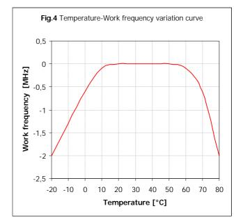
5V supply, RF 868,3 MHz, -100dBm input
