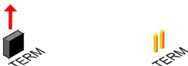
If different cable wiring topologies (tree, star, loop, ...) are used, place a jumper on the end module of the longest cable only, NOT on each end point.
