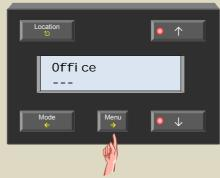
19. Select the sensor in the passage (to set up the differential thermostat) with the  $\uparrow$  or  $\downarrow$  button.
