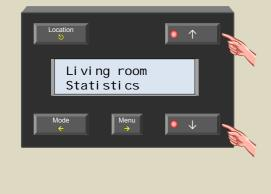
4. Select the statistics menu with the → button. The display shows the minimum temperature.
