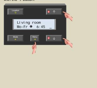
10.Set the mode (comfort, day, night or anti-freeze mode) with the ↑ or ↓ button and confirm with the →button.
