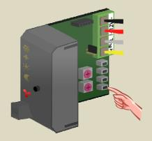
12. Set the address of the relay module back to its original value.
