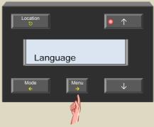
14. Scroll through the configuration menu using the ↑ or ↓ button until the 'Link wake up' item appears.
