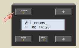
2. Set the heating (or AC) to anti-freeze or night mode using the 'Mode' button.
