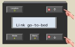
7. Select the link go to bed menu with the → button. As a confirmation, the relay of channel 1 is energised.
