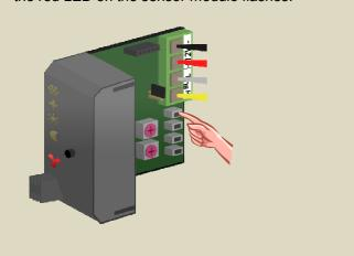
6. Set the address of the relay module back to its original value.
