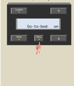
8. Confirm with the → button. The relay is de-energised.
