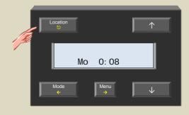
10. Set the address of the relay module back to its original value.
