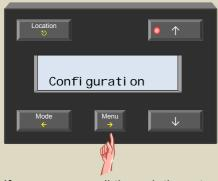
If necessary scroll through the extended menu using the ↑ or ↓ button until the 'Configuration' item appears.
