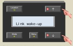
Select the link wake up menu with the → button. As a confirmation, the relays of the window shutter modules are energised.
