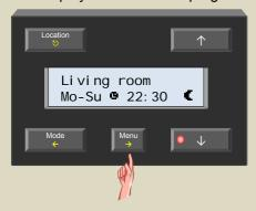
4. Scroll through the program using the ↑ or ↓ button until the instruction that needs to change is shown.
