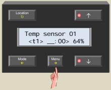
6. Change the hour of the first time frame with the ↑ or ↓ button and confirm with the → button.
