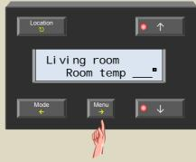
7. Enter the temperature as measured with a different thermometer using the  $\uparrow$  or  $\downarrow$  button.
