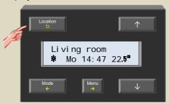
Press and hold the 'Menu' button for ±4 seconds to open the extended menu. Enter the PIN code if necessary.
