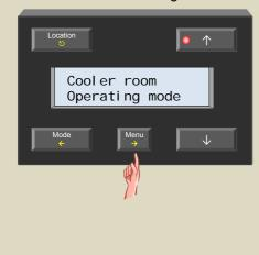
5. Scroll through the sensor settings menu using the ↑ or ↓ button until the 'Diff. Sensor' item appears.
