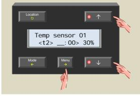
9. Change the hour of the second time frame with the ↑ or ↓ button and confirm with the → button.
