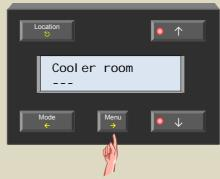
7. Select the second sensor of the differential thermostat using the  $\uparrow$  or  $\downarrow$  button.
