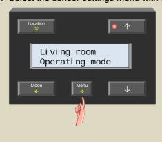
5. Scroll through the sensor settings menu using the ↑ or ↓ button until the 'Temp calibration' item appears.
