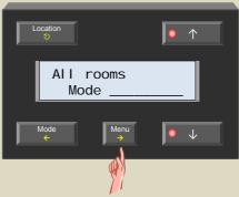
6. Change the mode to heating or cooling using the ↑ or ↓ button.
