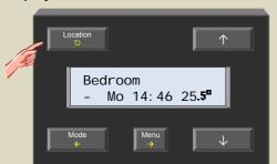
21. Press and hold the 'Menu' button for ±4 seconds to open the extended menu.
