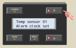
3. Select the alarm set menu with the → button. The alarm-indication flashes.
