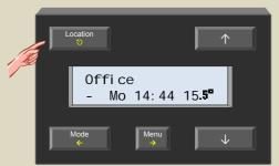
14. Press and hold the 'Menu' button for ±4 seconds to open the extended menu.
