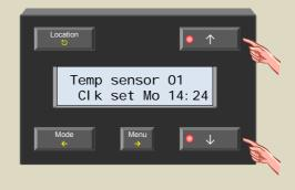
9. Confirm with the → button to start the clock from the set time.
