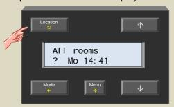
Press and hold the 'Menu' button for ±4 seconds to open the extended menu.
