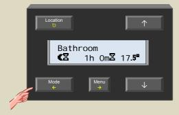
To indicate that temporary mode (sleep timer) is enabled, the LED on the 'Mode' button starts flashing and the display shows an hourglass. The indication LEDs on the sensor module also will flash.
