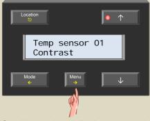
4. Scroll through the display menu using the ↑ or ↓ button until the 'Backlight' item appears.
