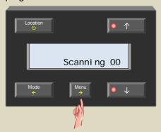
6. Once the search process is completed, the first of the connected temperature sensors is shown on the display.
