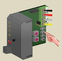
Press and hold the third push button (DAY) of the second temperature sensor until the relay is energised and the red LED on the sensor module flashes.
