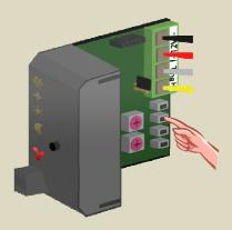
7. Press and hold the third push button (DAY) of the third temperature sensor until the relay is energised and the red LED on the sensor module flashes.
