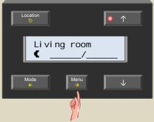
7. Use the ↑ or ↓ button until horizontal lines are displayed in the data entry fields.
