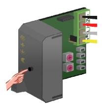
When the comfort, day or night mode LED is flashing, the sensor module is set temporarily (sleep timer) to the indicated mode. During this time the program is ignored
