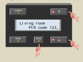
9. Change the last number of the PIN code with the ↑ or ↓ button and confirm with the → button.
