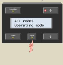
5. Scroll through the sensor settings menu using the ↑ or ↓ button until the 'Upper cool temp' item appears.
