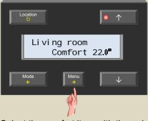
4. Select the comfort item with the → button. The desired comfort temperature starts flashing.
