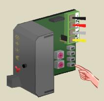
6. Set the address of the first relay module back to its original value.
