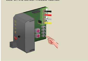
6. Set the address of the relay module back to its original value.
