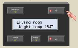
12.Select the night item with the → button. The desired night time temperature starts flashing.
