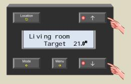
3. Return to normal display by pressing the ♥ or ← button or simply wait for ±5 seconds without touching any button.
