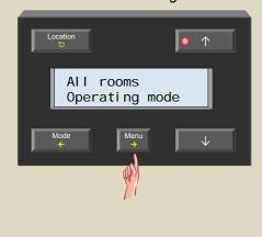
5. Scroll through the sensor settings menu using the ↑ or ↓ button until the 'Low temp. alarm' item appears.
