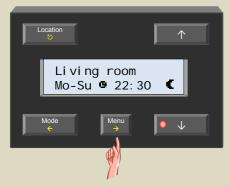
4. Scroll through the program using the ↑ or ↓ button until the instruction that needs to be removed is shown.
