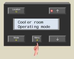
11.Scroll through the sensor settings menu using the ↑ or ↓ button until the 'Diff. sensor' item appears.
