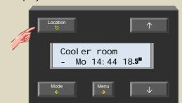
8. Press and hold the 'Menu' button for ±4 seconds to open the extended menu.
