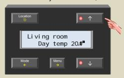
Select the day item with the → button. The desired daytime temperature starts flashing.
