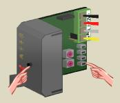
7. Press and hold the pushbutton on the front panel of the third temperature sensor and simultaneously press and hold the lowest push button (HEAT) until the relay is energised and the red LED on the sensor module flashes. First release the lowest push button (HEAT) followed by the push button on the front panel.
