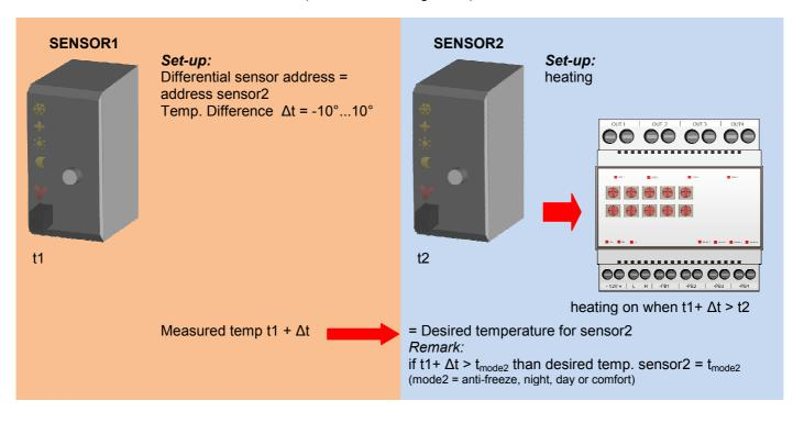
Schematic overview differential thermostat (sensor2 in cooling mode):
