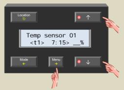
Set the brightness for the first time frame with the ↑ or ↓ button and confirm with the → button.
