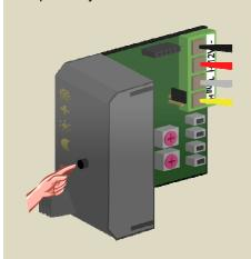
2. Set the MODE and TIME1 rotary switches for channel 1 of the second relay module to '0' (instant control).
