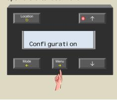
12.If necessary scroll through the extended menu using the ↑ or ↓ button until the 'Configuration' item appears
