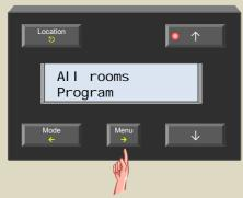
3. Scroll through the extended menu using the ↑ or ↓ button until the 'Sensor settings' item appears.
