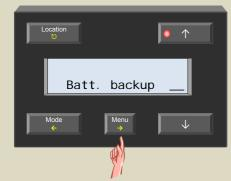
6. Enable the battery backup watchdog when a battery is inserted or disable it when no battery is present using the ↑ or ↓ button.
