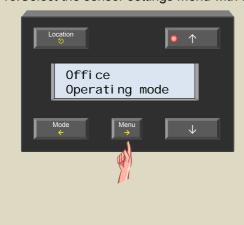
17. Scroll through the sensor settings menu using the ↑ or ↓ button until the 'Diff. sensor' item appears.
