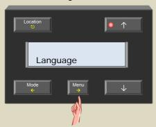
6. Scroll through the configuration menu using the ↑ or ↓ button until the 'Link go-to-bed' item appears.
