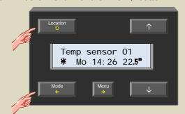
The **4** symbol is no longer visible on the display to indicate that the alarm function is disabled.
