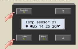
The **\$** symbol indicates that the alarm function is activated.
