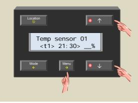
11. Set the brightness for the second time frame with the  $\uparrow$  or  $\downarrow$  button and confirm with the  $\rightarrow$  button.
