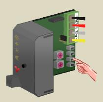
6. Set the address of the second relay module back to its original value.
