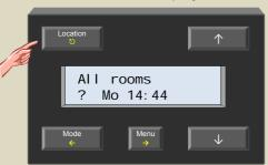
2. Press and hold the 'Menu' button for ±4 seconds to open the extended menu.
