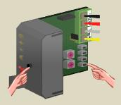
8. Set the address of the first relay module back to its original value.
