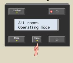
5. Scroll through the sensor settings menu using the ↑ or ↓ button until the 'Temp difference' item appears.
