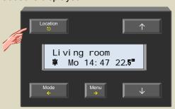
Press and hold the 'Menu' button for ±4 seconds to open the extended menu. Enter the PIN code if necessary.
