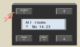
Set the heating to anti-freeze mode using the 'Mode' button.
