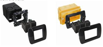
It is also possible to use a 2- or 3-module wide frame with cover plate from the BTicino Light or Light Tech series. The module must be pushed into the build-in frame from the front.
