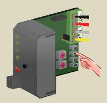
8. Set the address of the first relay module back to its original value.
