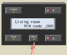
Change the first number of the PIN code with the ↑ or ↓ button and confirm with the → button.
