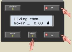
Use the ↑ or ↓ button to set the time reference (exact, relative to wake-up or go-to-bed time) on which the instruction needs to be executed. Confirm with the → button.
