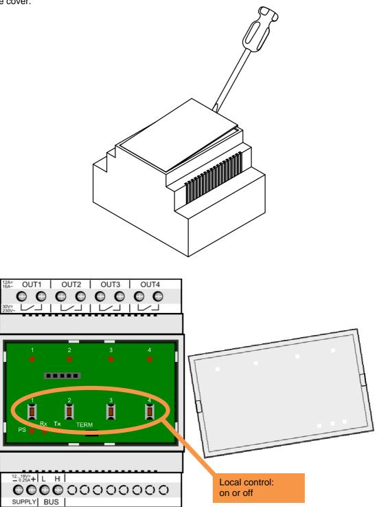
The relay module features 4 non-voltage NO contacts wich allow you to switch mains-voltage (230V) and low-voltage (12 or 24V) consumers.
