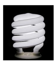
A spiral-type integrated compact fluorescent lamp, with combined tube and electronic ballast. This style has slightly reduced efficiency compared to tubular fluorescent lamps, due to the excessively thick layer of phosphor on the lower side of the twist. Despite this, it has become one of the most popular types among consumers since its introduction in the mid 1990's.
