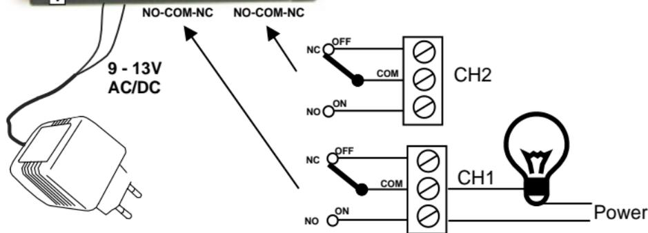
Any type of power can be used, AC or DC, the maximum current is 130mA. The polarity is not important
