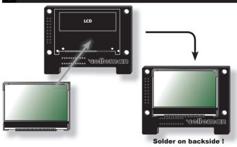
Be careful when soldering the LCD connections.
