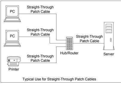
These are generally used for connecting computers to hubs (routers or switches) or simply between a PC and a wall socket (which eventually connects to a hub).
