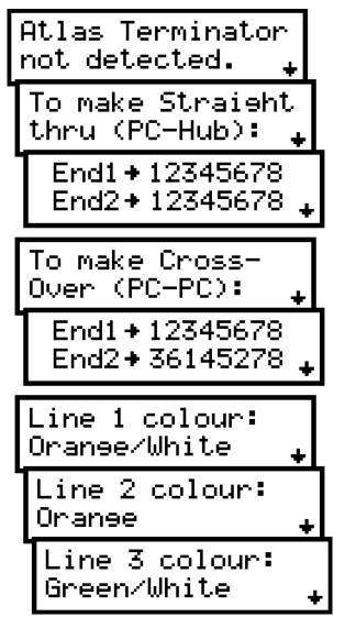
$\leftarrow$  First the unit confirms the connection patterns for the two most common cable configurations (Straight-Through Patch cables and Crossover cables).
