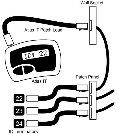
These special terminators can be used in exactly the same way as the standard (non-identified) terminators. They are automatically recognised by the *Atlas IT*
