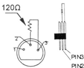
A DMX terminator is recommended for installations where the DMX cable has to run a long distance or is in an electrically noisy environment (e.g. discos). The terminator prevents corruption of the digital control signal by electrical noise. The DMX terminator is simply an XLR plug with a 120Ω resistor between pins 2 and 3, which is then plugged into the XLR output socket of the last device in the chain.
