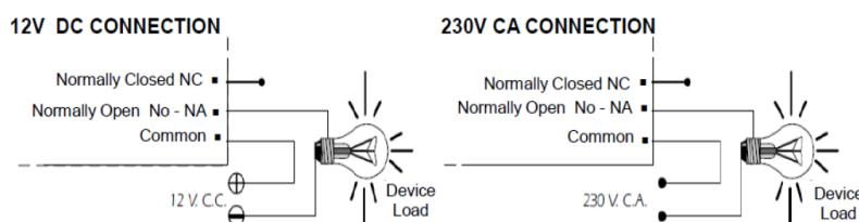
**OUTPUT CONSIDERATIONS :** During the operation of the circuit, and depending on its load, a fluctuation or incorrect operation of the output may occur. If this occurs, install a non-sparking circuit between the two relay contacts used in the connection.
